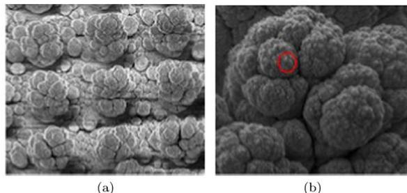
FIG. 2 (color online). Scanning electron microscope images of the snow targets. Total width shown is 1000  $\mu\text{m}$  (a) and 100  $\mu\text{m}$  (b). Red circle represents the laser spot.
