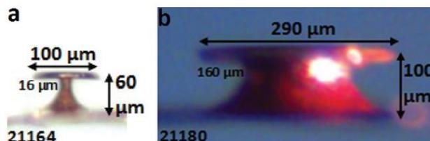
FIG. 4. (Color) Target pictures (to scale): the OD of the various necks ranged from (a) 11  $\mu\text{m}$  (shot 21164) to (b) 160  $\mu\text{m}$  (shot 21180).
