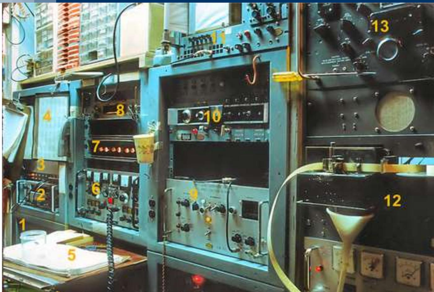
*Some of the equipment inside Transit satellite tracking station 019. 1. Automatic Control Unit, 2. timer-counter, 3. Time burst detector, 4. time conversion chart, 5. satellite ephemeris, 6. tracking receiver, 7. time display, 8 Header-Tailer programmer, 9. Digitizer and main clock, 10. master oscillator, 11. strip chart recorder, 12. paper tape punch, 13. short wave receiver. Out of sight: VLF receiver, refraction correction unit, backup battery system, power supplies, AC voltage regulators.*
